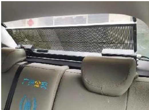
4. Place the power cord in the seat gap.
