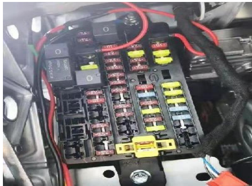
5. Connect the fuse to the corresponding insurance seat.
