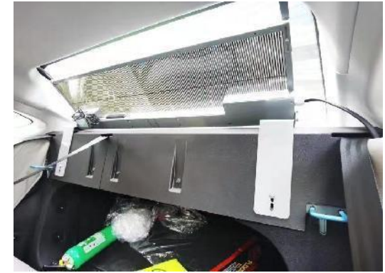
3. Put the bracket into the rear seat gap. Then connect the power cord.
