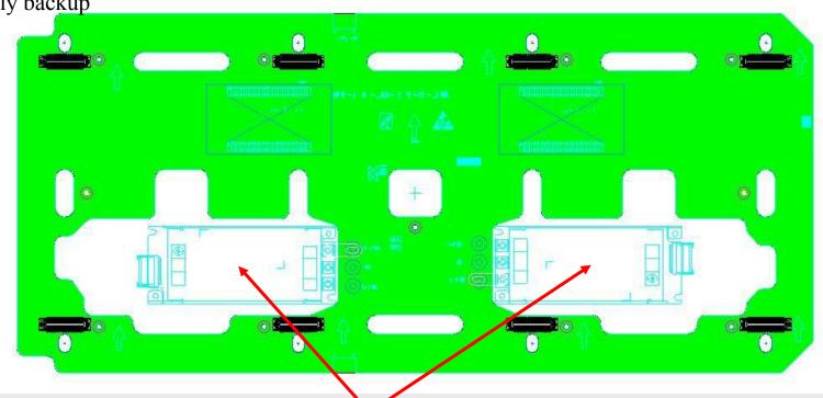
It supports dual power supply backup. A single-point fault does not affect the overall operation and is suitable forhighreliability scenarios (such as command centers and studios)
