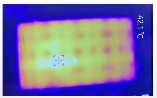
The system card is placed on the back of the box, and the power supply is designed close to the die-cast box, which improves the heat dissipation efficiency, avoids the temperature rise of the module caused by excessive heat generation of the system card and the power supply, distributes the heat more evenly, and eliminates the local...local of the module caused by heat "Slightly bluish or slightly reddish" Phenomenon
