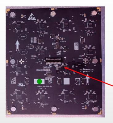
The pin definition of the lamp board connector is a foolproof design.100%Eliminate the risk of board burning caused by reverse installation, even for beginners.Zero installation errors.
